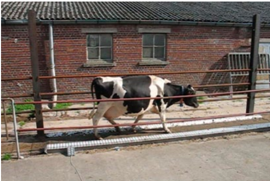
Figure 1 Cow walking on a 6 m long instrumented walkway to measure the gait kinematics at ground contact level.
